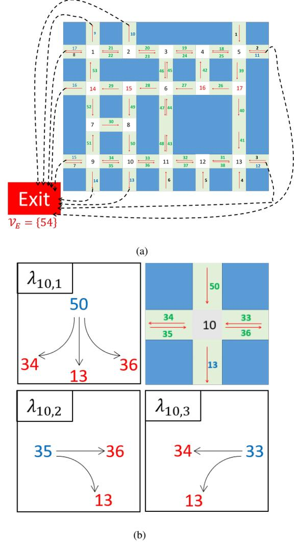
Fig. 1: (a) Example NOIR with 53 unidirectional roads. (b) Three possible movement phases at junction  $10 \in \mathcal{W}$ .
